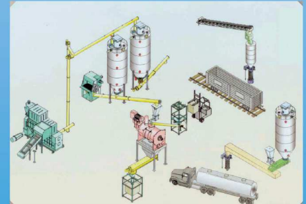
Mechanical & Pneumatic Conveying System
